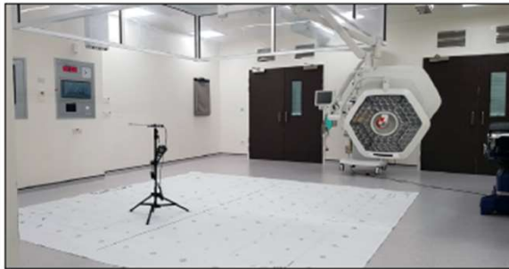
UCV canopy entrainment test
